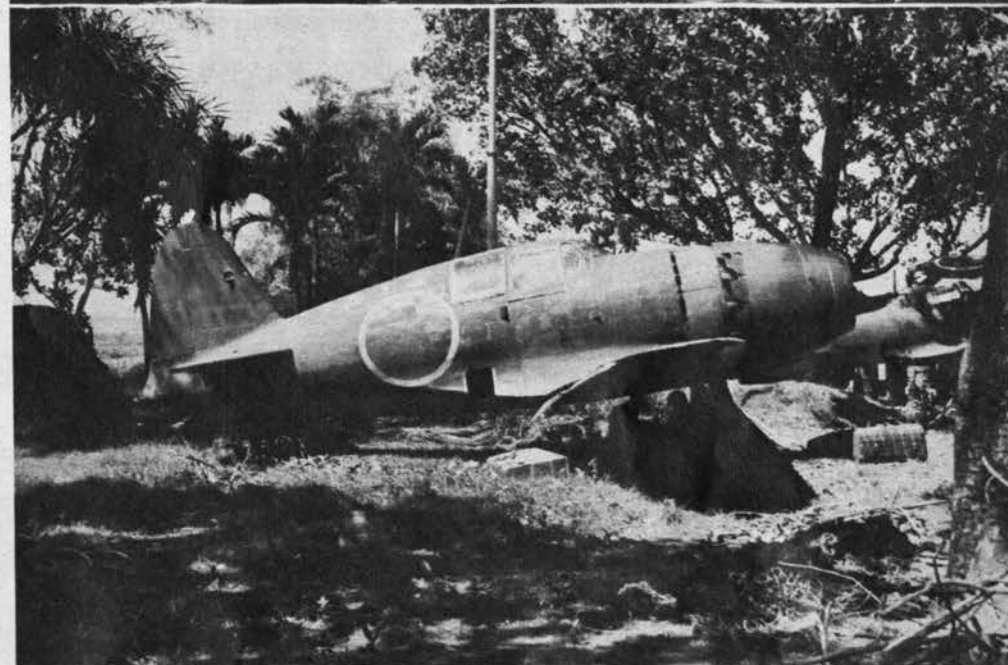
Fat, curved lines of Jack's turtleback fuselage are broken by the cockpit fairing. The round, radial nose projects beyond stubby wing like the end of a beer keg.
